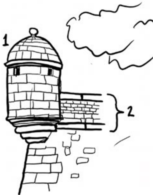
Figure 4: A typical bastion salient showing 1. the corbelled Echaulette and 2. the decorative Cordons and Tablette of the wall.
